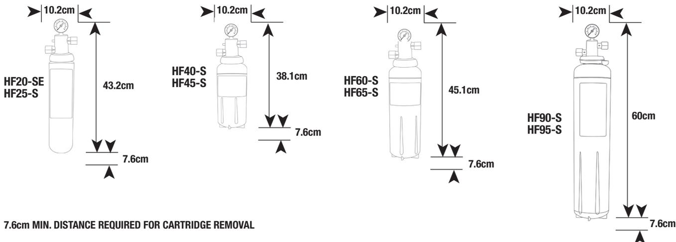
7.6cm MIN. DISTANCE REQUIRED FOR CARTRIDGE REMOVAL
